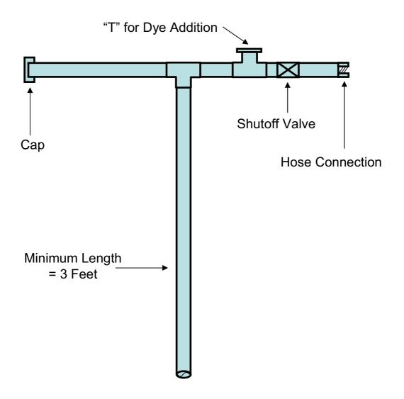
To be constructed of 3/4 or 1 inch rigid steel pipe
