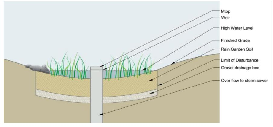
\*Note: Rain Garden does not have an under drain.
